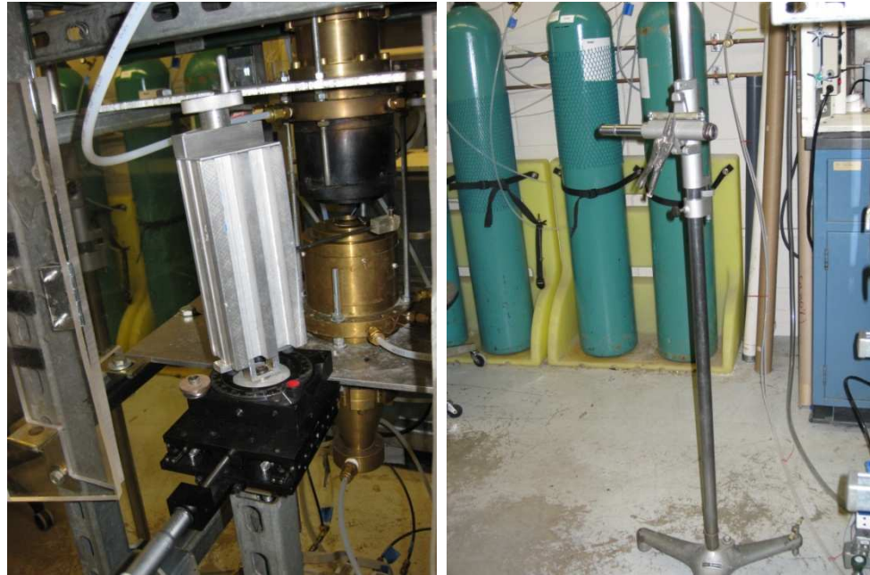
Figure 2.5 Three axis translator (left) and cathetometer (right).
