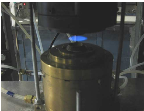
Figure 2.1 Actual image of CDF with methane flat flame.
