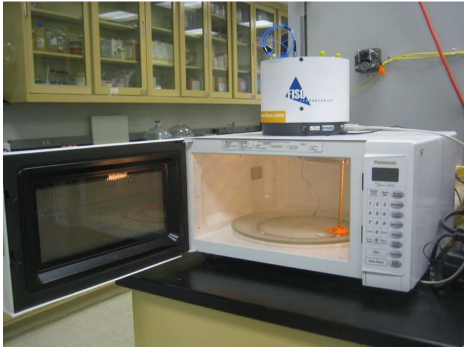
a. With only one fiberoptic probe connected. Not showing connection to computer.
