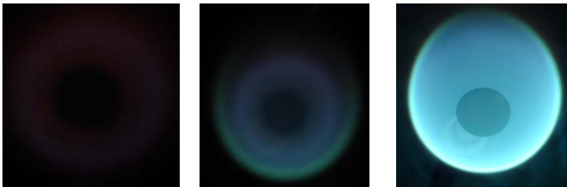
Figure B.2. Spherical diffusion flames of different fuels. a) Pure hydrogen. b) Hydrogen/methane mixture. c) Pure methane
