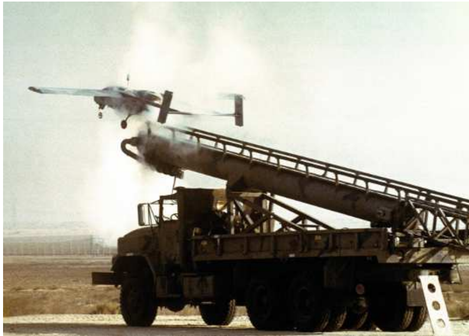
Figure 4.1: A Pioneer UAV is catapulted from a launching rail set up atop an M-814 5-ton cargo truck during a test in support of Operation Desert Shield in 1991 [49].
