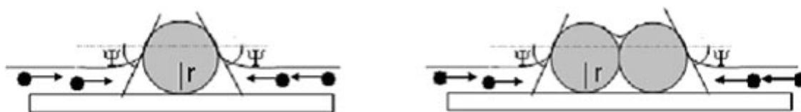
Figure 5.8: Theoretical model showing agglomeration of polystyrene particles and effect of lateral capillary forces on \text{TiO}_2 particles
