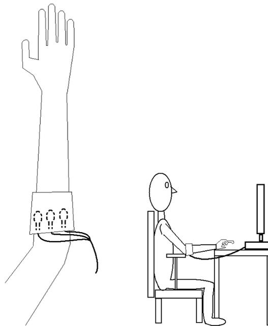
Figure 1 – The PAMI device. Worn on an upper limb as in typical use (left), and shown during training (right). Note the distribution of sensors about the forearm, and the support of the elbow and wrist during training.
