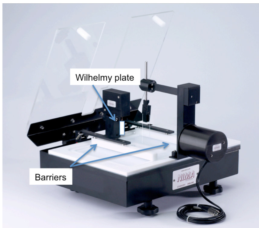
Figure 1-10. Instrumental setup of Langmuir-Wilhelmy balance
