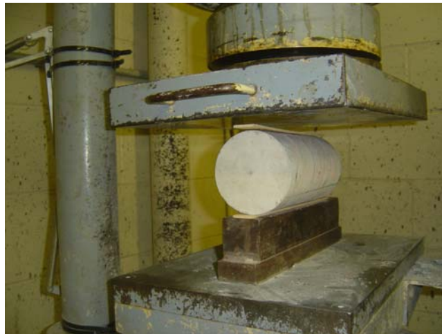
Figure 3-8 Splitting Tensile Strength Test Setup
