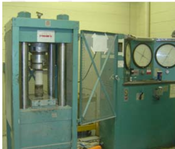
Figure 3-7 Forney 1-Million Pound Compression Machine
