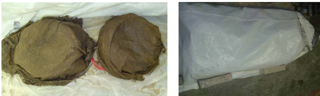
Figure 3-6 Ring Specimens Covered with Burlap and Sealed with Polyurethane Sheet
