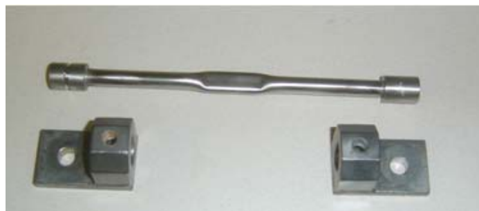
Figure 3-11 Geokon Model 4000 VWSG's and Modified Mounting Blocks
