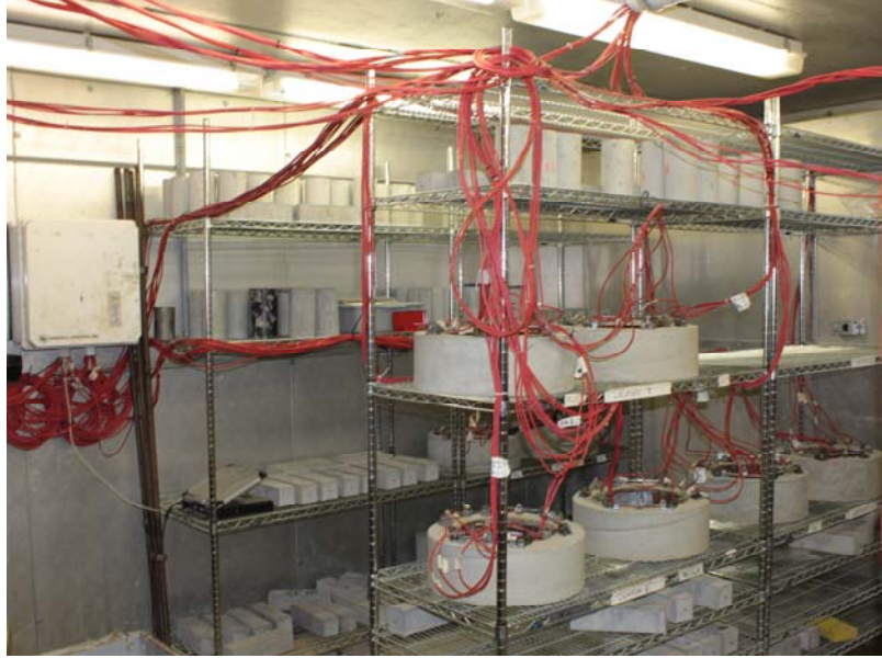
Figure 3-17 Ring Specimens Monitored in Environmental Chamber
