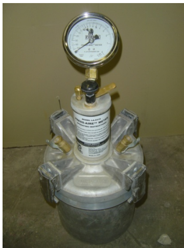
Figure 3-5 ASTM C – 231 Type B Pressure Meter
