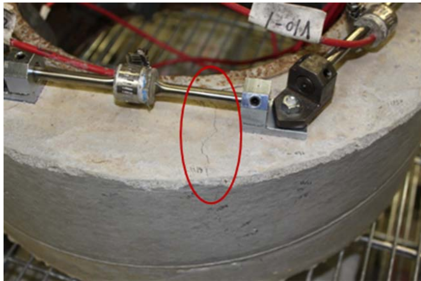
Figure 4-28 Full Depth Shrinkage Crack Observed on G1M3 Ring Specimen 1
