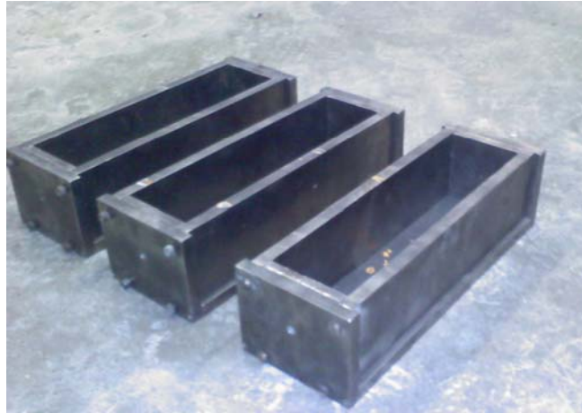
Figure 3-10 Steel Free Shrinkage Molds
