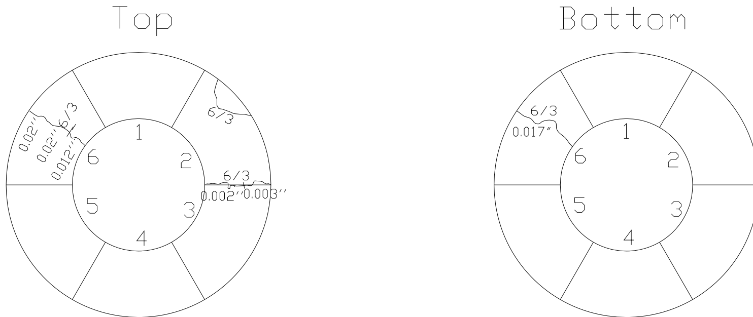
Figure 4-38 G2-M3 Crack Drawings for Ring Specimen 1, Side View (Top Figure) and Top-Bottom Views (Bottom Figure)
