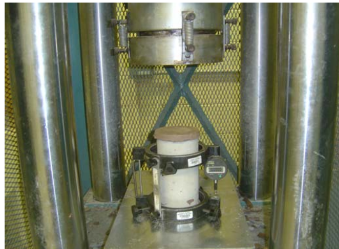
Figure 3-9 Modulus of Elasticity Test Setup
