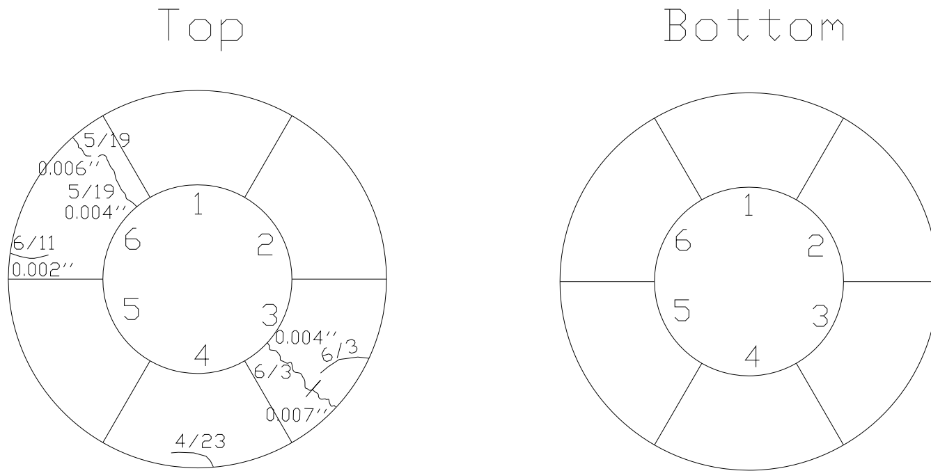
Figure 4-39 G2-M3 Crack Drawings for Ring Specimen 2, Side View (Top Figure) and Top-Bottom Views (Bottom Figure)
