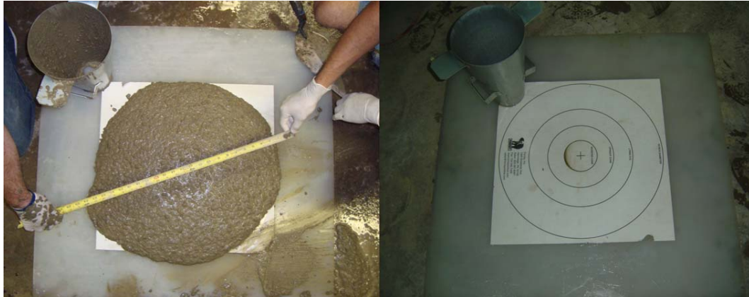
Figure 3-2 Slump Flow Testing (ASTM C1611M-05)
