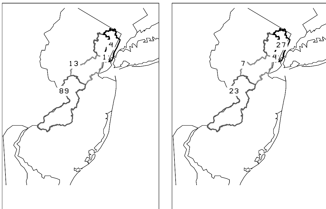
FIG 1.4. PSE&G total plant damage observations (left) and corresponding Thunderstorm model prediction (right) for 9 June 2009.
