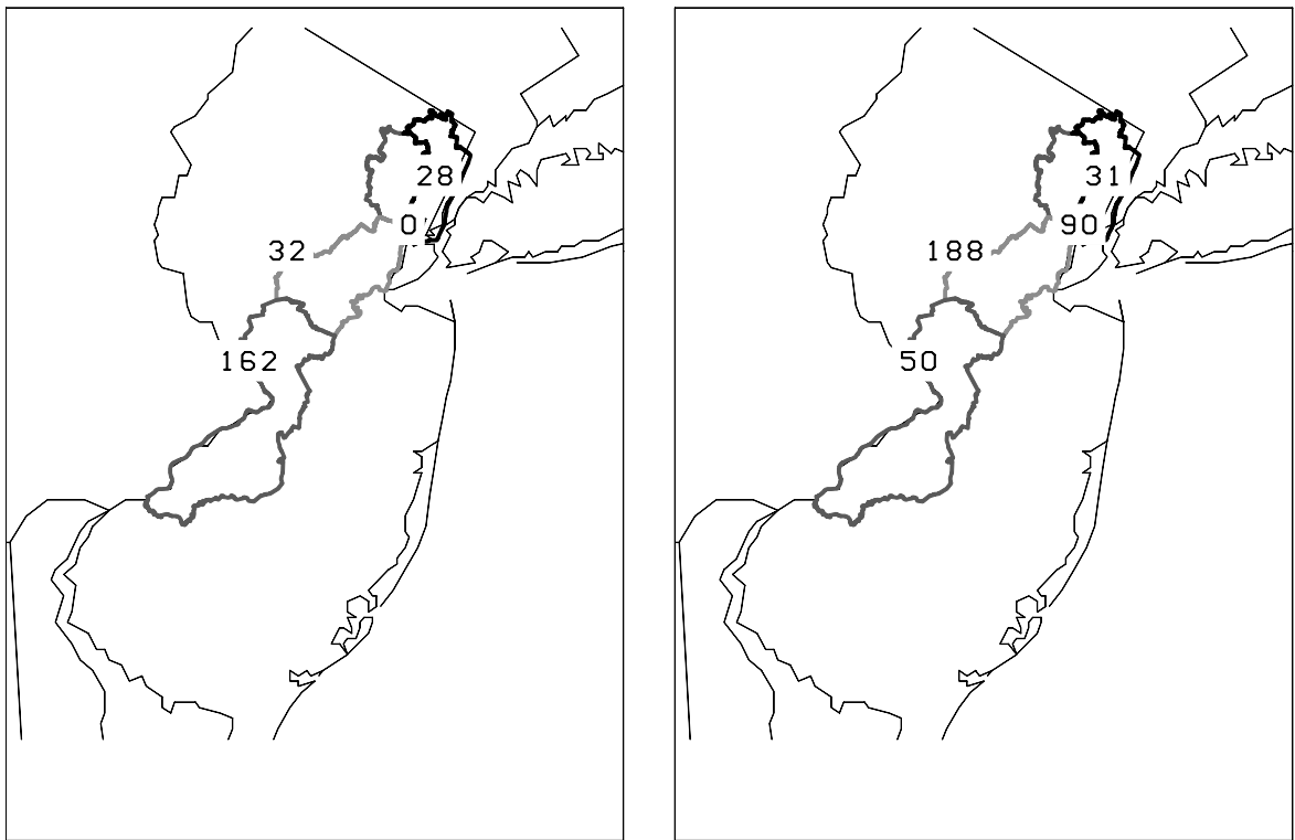
FIG 2.2. PSE&G plant damage observations (left) and Thunderstorm storm mode model prediction (right) for 26 July 2009.
