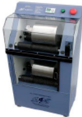
Figure 4.13 – Picture of the Micro-Deval Test Apparatus
