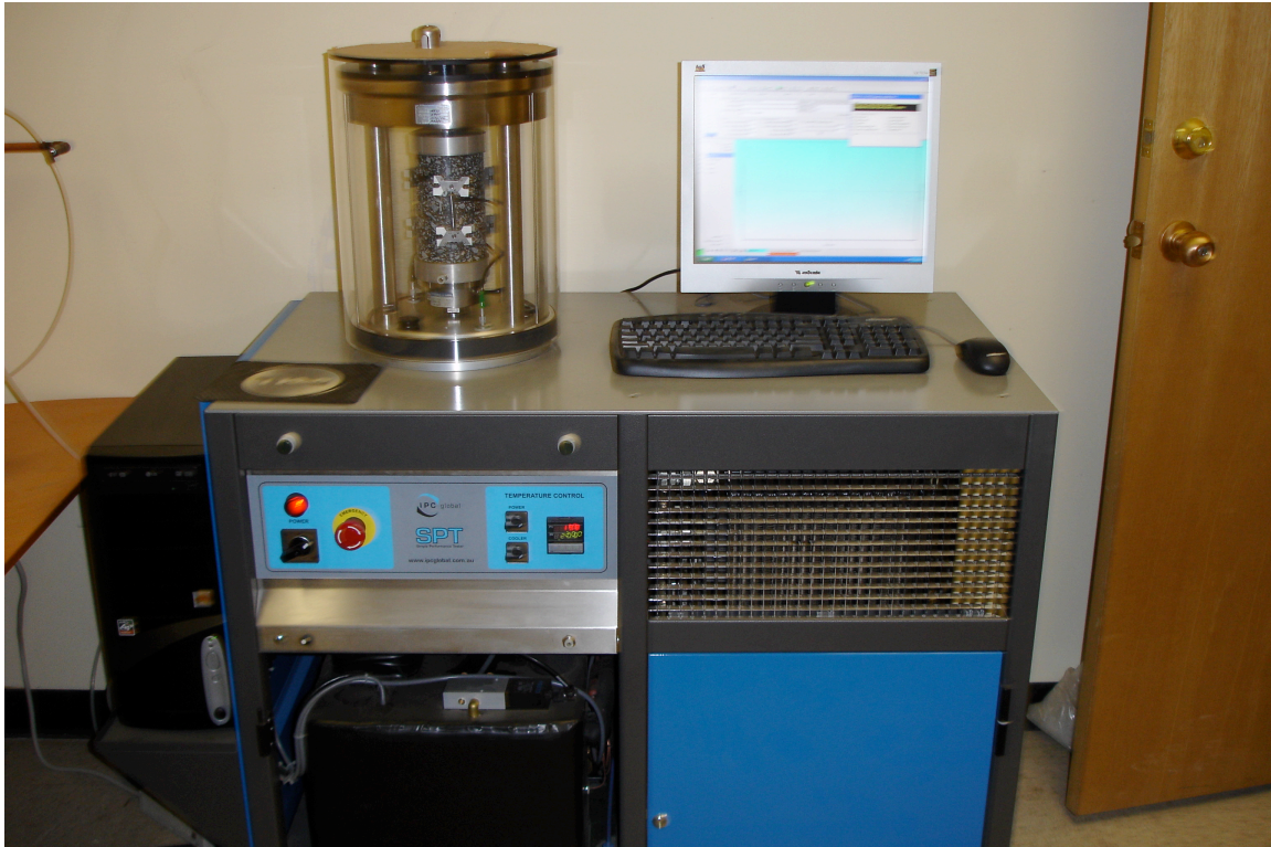
Figure 6.18 – Asphalt Mixture Performance Tester (AMPT) Used in Study
