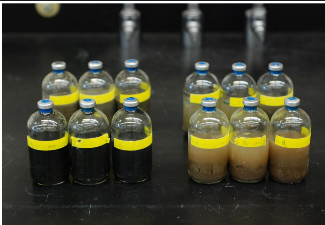
Figure 4.1.1 Photograph of different treatments during TEST 1, Degradation of Paper Saturated with Inhibitors I . Note color differences where darker bottles produce greater amounts of biogas and methane than lighter colored bottles.
