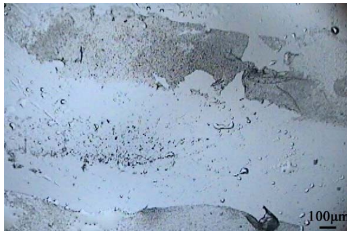
Figure 3.13. Microscope View of Wet Dermis Residue on Sapphire Window (20 pulses/ \mu\text{m} & 2.5 \mu\text{J} , 40X)
