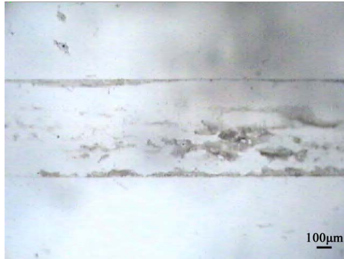
Figure 3.12. Microscope View of Separated Wet Dermis Layer on Sapphire Window after 2 times Repeat with 20 \mu\text{m} Increase (40X).
