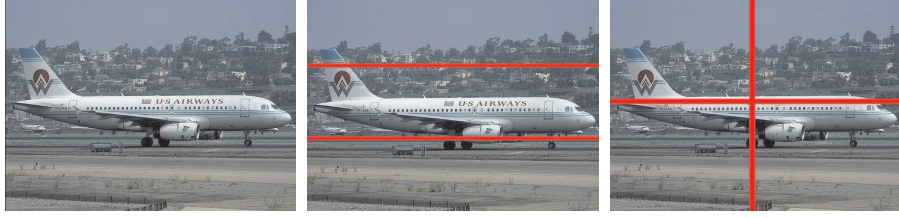
Figure 5.2: The spatial pyramids for the distance measure based on the appearance descriptors. Three levels of spatial pyramids for the appearance features are: 1 \times 1 (whole image, l = 0 ), 1 \times 3 (horizontal bars, l = 1 ), 2 \times 2 (image quarters, l = 2 ).
