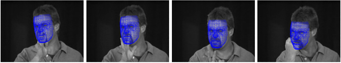
Figure 3.7: Results of sign language tracking sequence using ASM, KLT and edge tracking.
