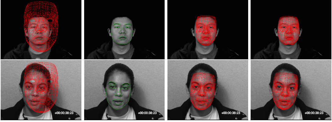
Figure 3.5: Automated model fitting and adaptation. Left to right: Before model fitting, ASM feature detection, Adjustment of rigid model parameters, Final fit after adjustment of nonrigid shape parameters.
