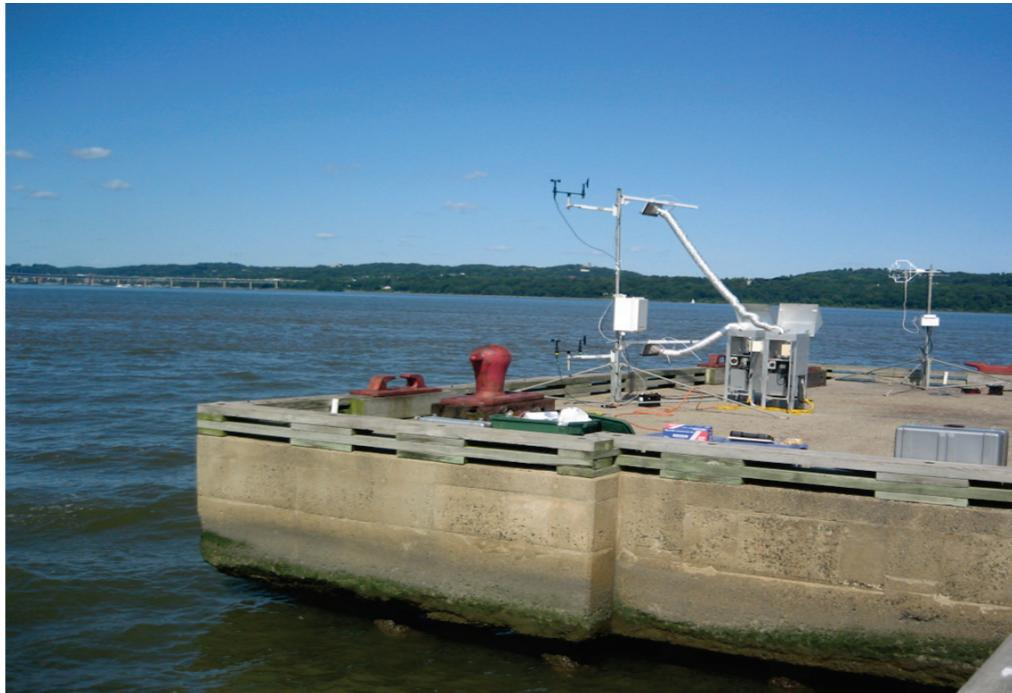
**Figure 2-2.** Air sampling apparatus on the peirmont pier at the Tappan Zee.
