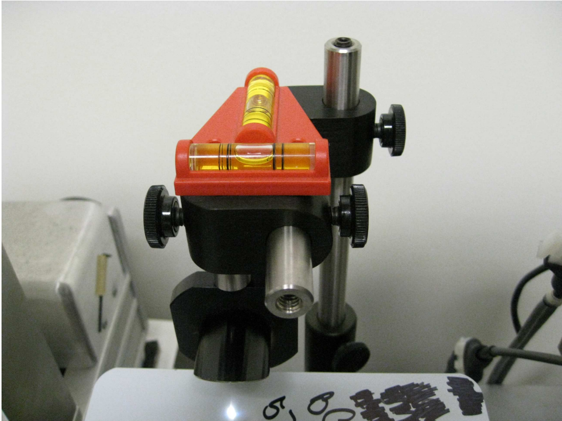
Figure A.8: To complete the alignment of the mirror, place the spirit level on the mirror mount and rotate the mount about its horizontal axis until the bubble is at the center of the tube.
