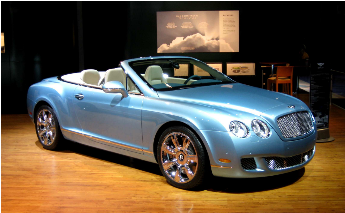
Figure 2.1: Appearance of an automotive coating. Metallic flakes present within the coating cause the blue finish of this car to show a change in brightness with viewing angle. The change in brightness enhances the visual appearance of the curved body of the car. The sparkle and texture of the finish further add to its dynamic appearance.
