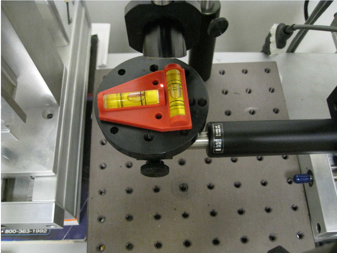
Figure A.9: Place the spirit level on the scanning stage and gently rotate the stage either using the mount that is fixed to it or the mount that attaches it to the stepper motor, or both until the bubble is at the center of the tube.
