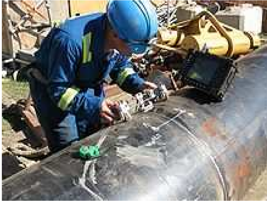
Figure 5.1: Application of non-destructive testing using ultrasonic waves
