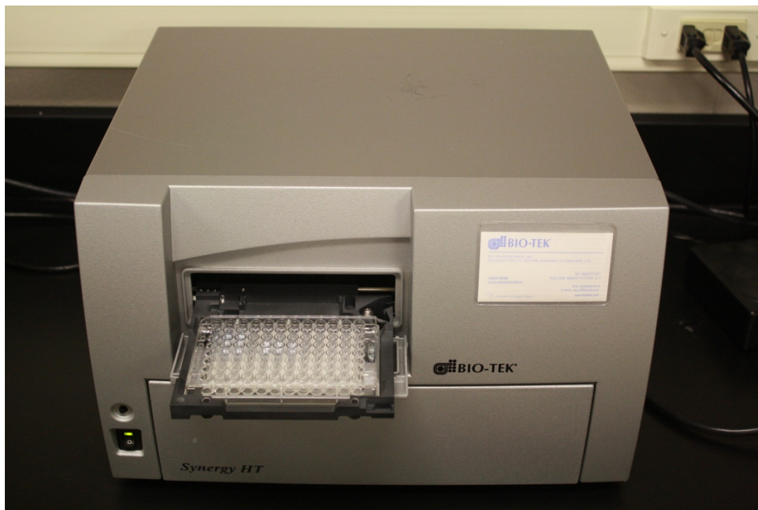
Figure 2.7: Bio-Tek spectrophotometer with 96-well plate used for measurement of TPC
