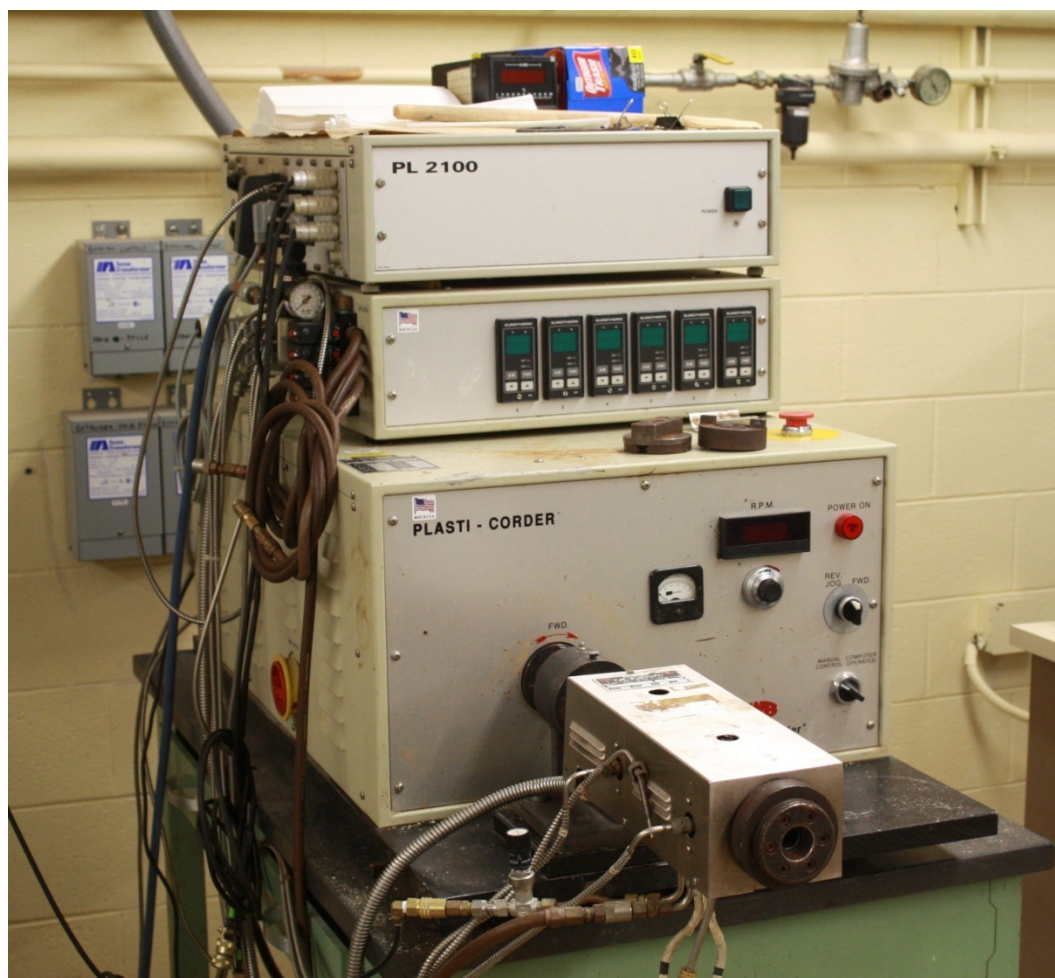
Figure 2.3: Brabender extruder in Rutgers, Food Science pilot plant
