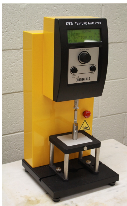
Figure 2.8: Brookfield Texture Analyzer (CT3) used for measuring breaking strength
