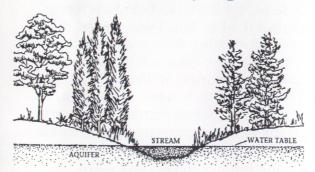
Beneath the surface of New Jersey's Pinelands is a vast quantity of water in the sand. This sand formation is called the Kirkwood-Cohansey Aquifer System and contains 17 trillion gallons of water. It supplies Pinelands communities with some of the purest drinking water in the world. It also feeds the rivers and streams of the Pinelands.
