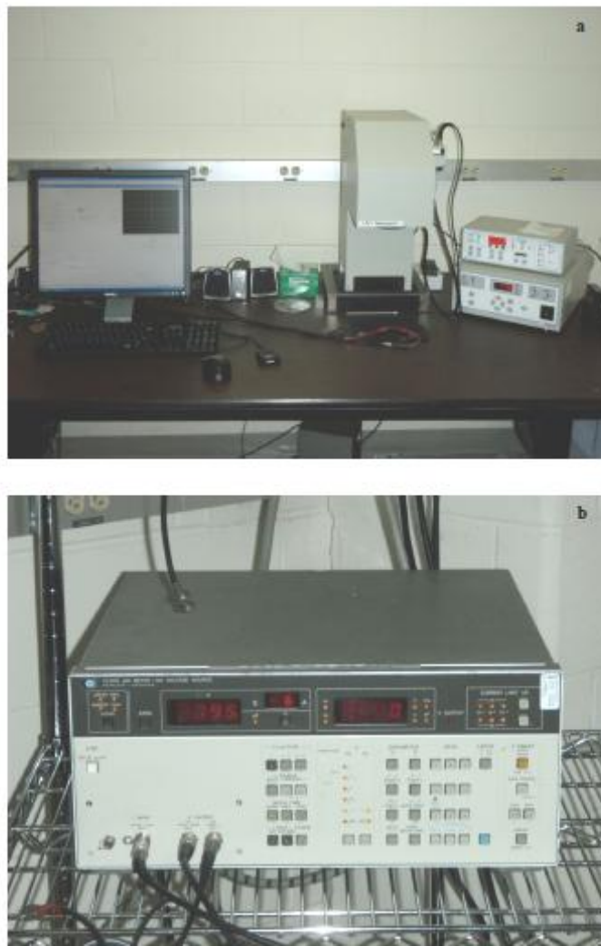
Figure 2.7: a. Newport solar simulator and computer and b. the voltage supply.
