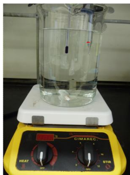
Figure 2-1. Apparatus for measuring clear point. Shea butter was expected to be filled in the apparatus up to the line on the pipett.
