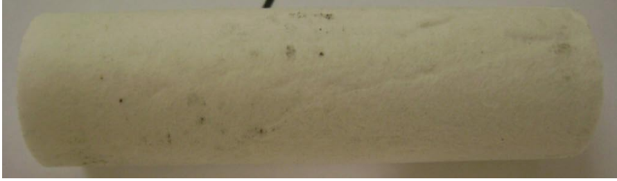
Figure 42: SEMTECH-D filter after use with three runs using the DPF & CCVS retrofits configuration.
