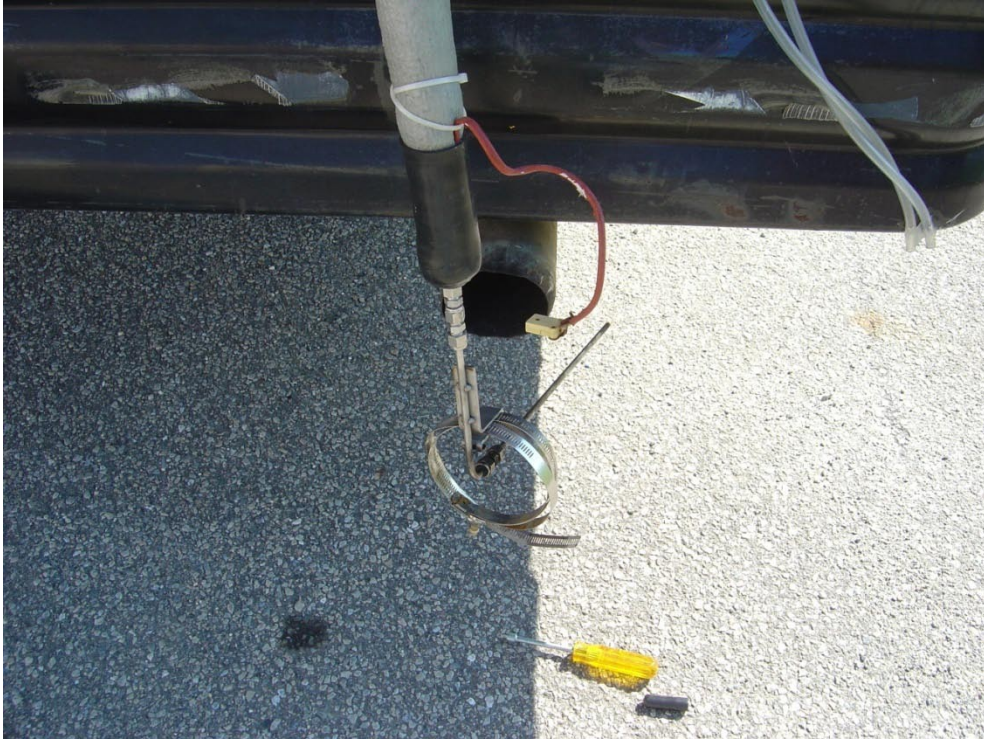
Figure 21: SEMTECH-D sampling tip before being inserted and secured to the tailpipe. Picture of the system taken for the final set of runs.
