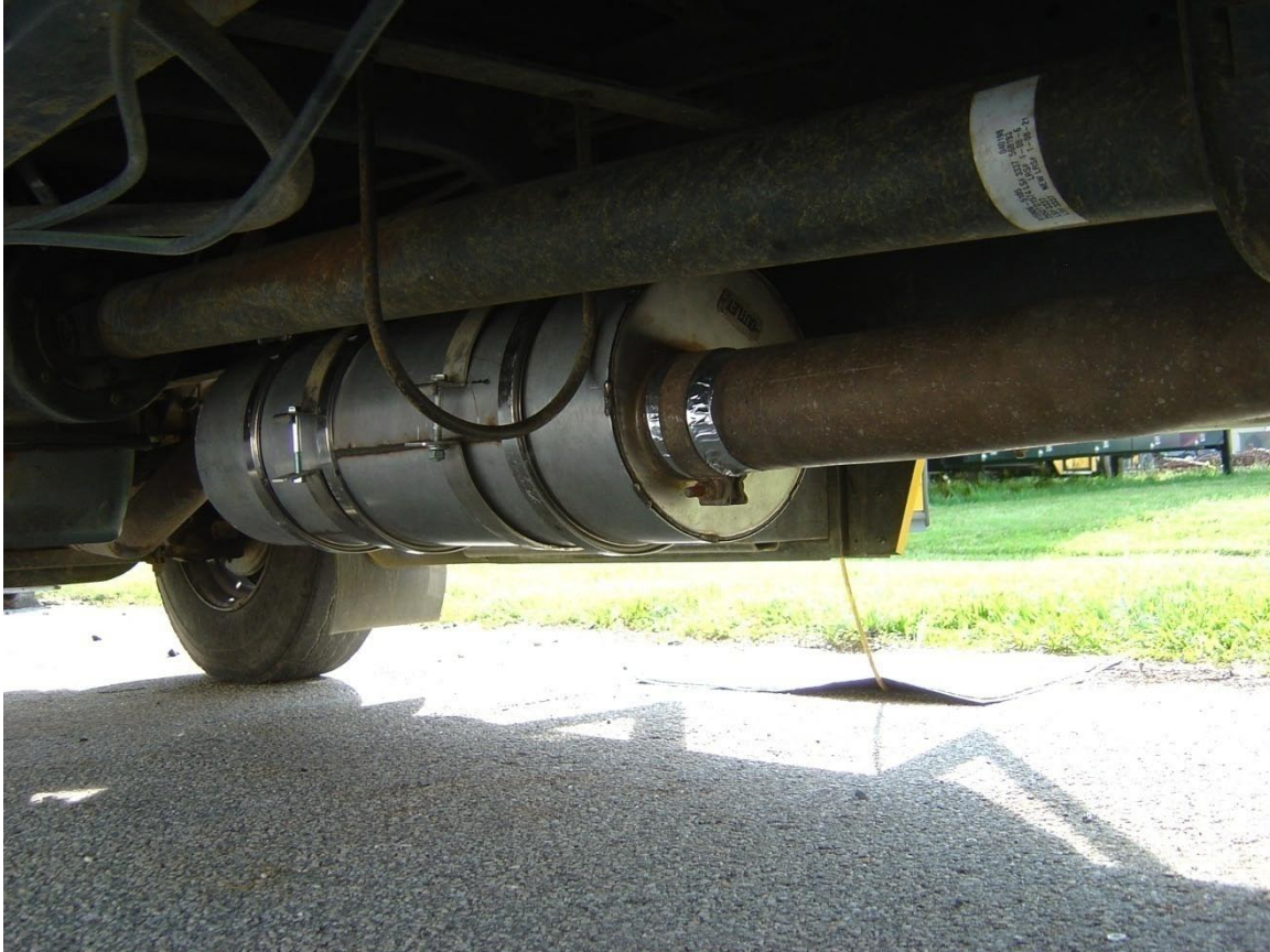
Figure 15: Johnson Matthey CRT, DPF, installed on the school bus.
