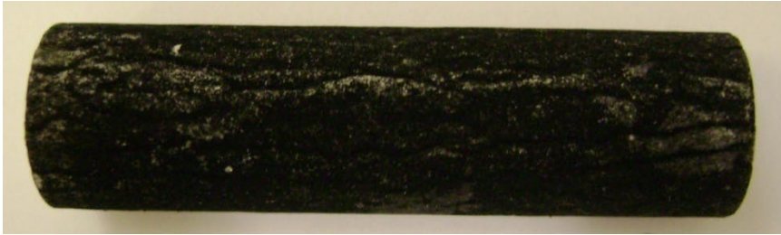
Figure 43: SEMTECH-D filter after three runs with the FTF and CCVS configuration.
