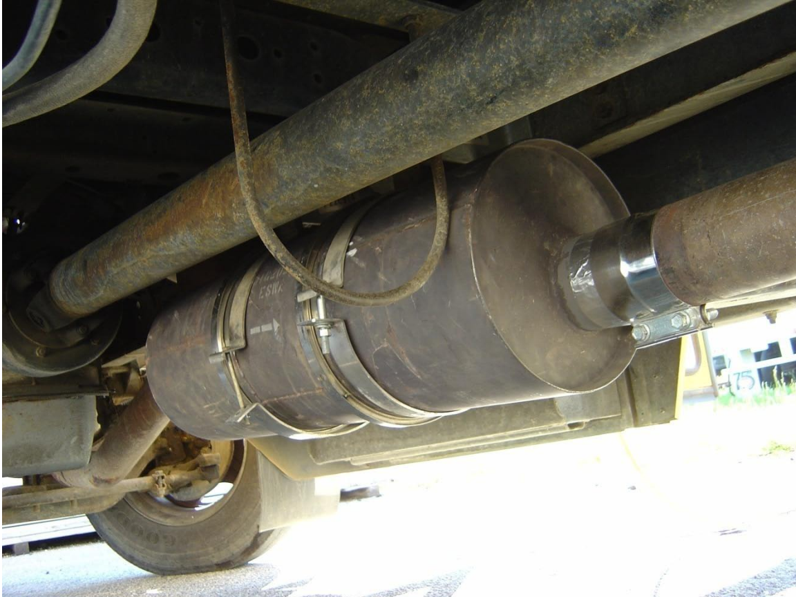
Figure 13: ESW Particulate Reactor (FTF) installed on the school bus.
