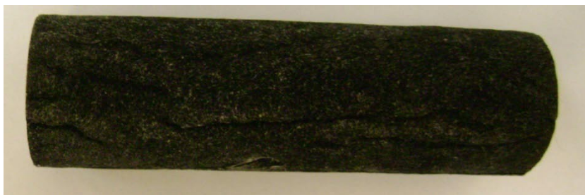
Figure 41: SEMTECH-D filter after use with three runs with no tailpipe retrofit for baseline condition.
