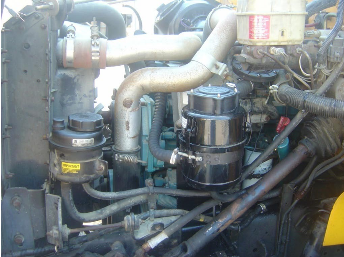
Figure 17: Donaldson Spiracle Crankcase ventilation system, CCVS, installed in the school bus tested. Picture taken prior the final set of runs.
