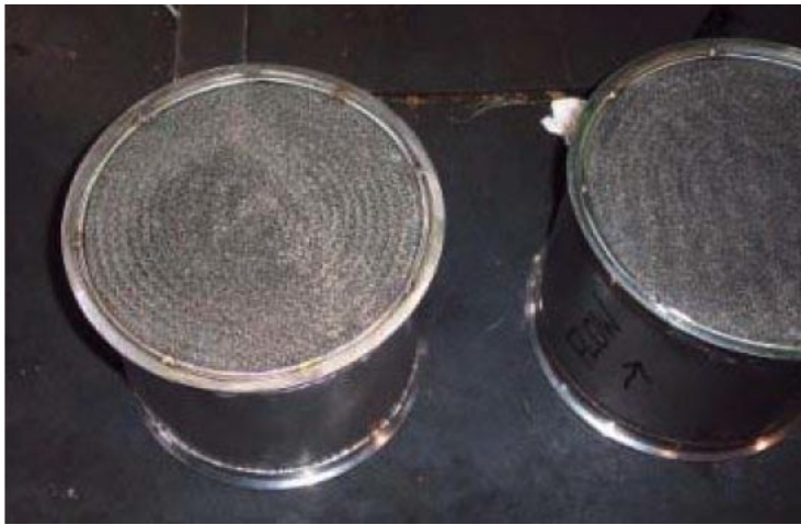
Figure 12: Internal component of the ESW Particulate Reactor®. Source: M.J. Bradley & Associates, Inc. (2006) 13 .
