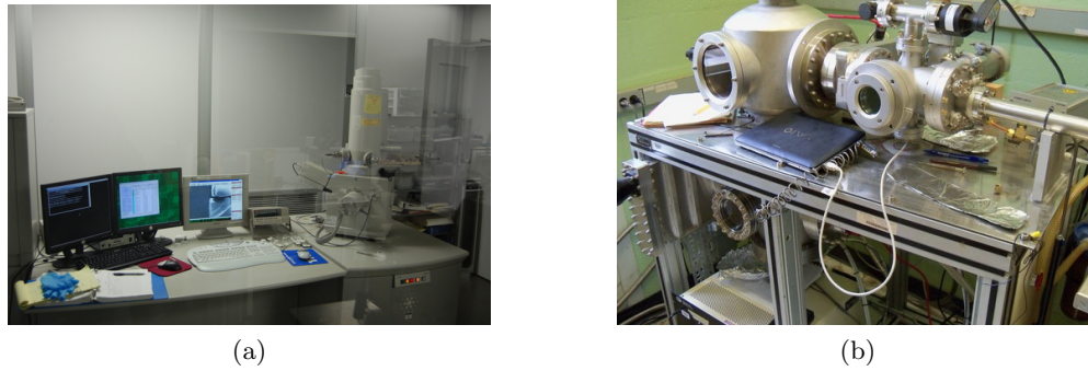
Figure 6.4: a , The FEI Sirion SEM in lithography mode. b , The metal evaporation chamber.
