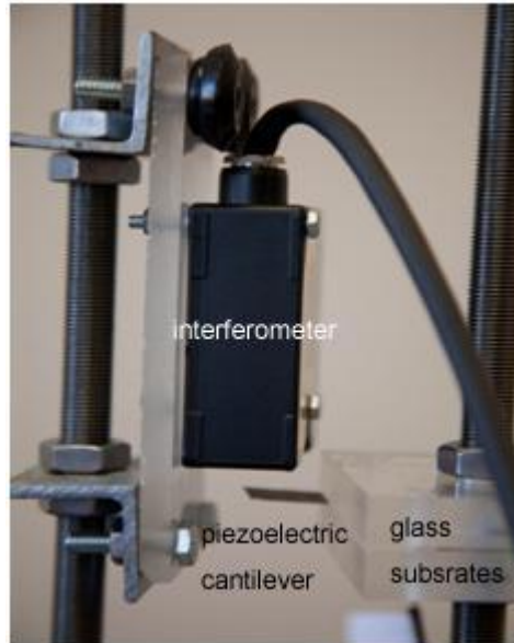
Figure 3.1 Illustration of the unimorph piezoelectric cantilever system, comprising of a cantilever, glass substrates, laser displacement sensor
