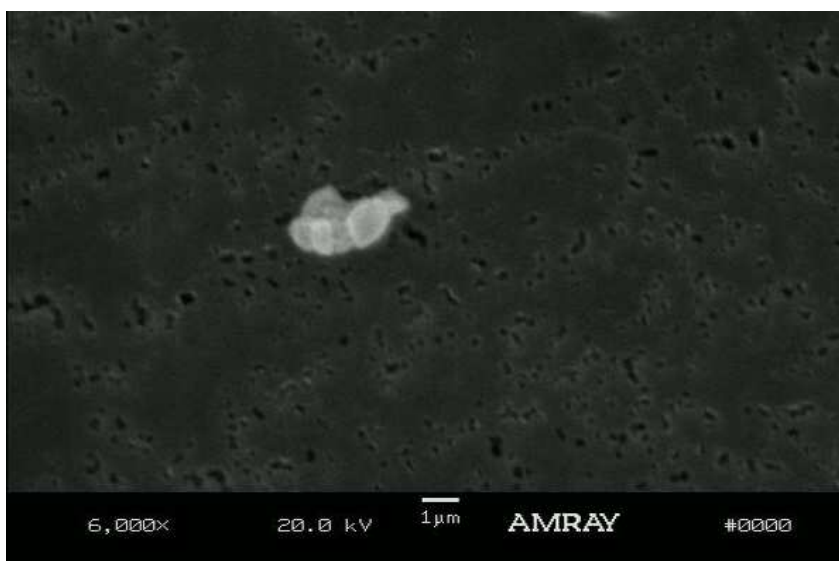
Figure 3-7: Representative SEM images of porous PCTE membrane after exposure to sheep's blood in a non-coated microdevice.
