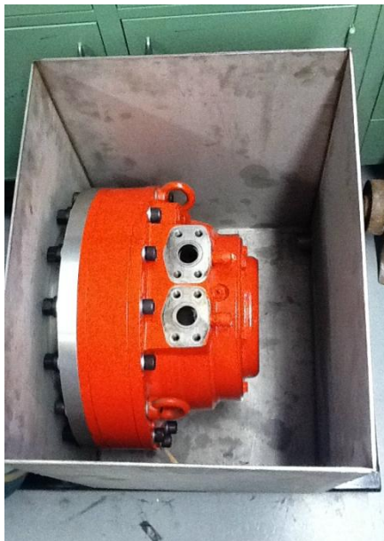
Figure 44: Hagglunds CA50-32 radial piston pump, top down view, installed in a sheet metal tank. Inlet and outlet ports are exposed on the top.
