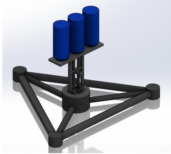
Figure 5: BioWAVE energy capture device rocks fore and aft, compressing fluid and generating electricity all at the source.
