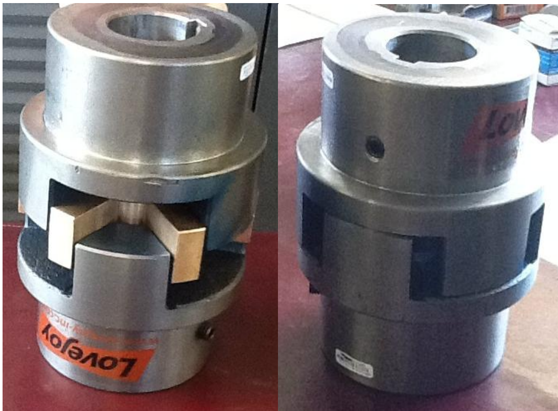
Figure 70: (Left) Lovejoy coupling fails to fully engage. (Right) Fully engaged coupler, without brass
