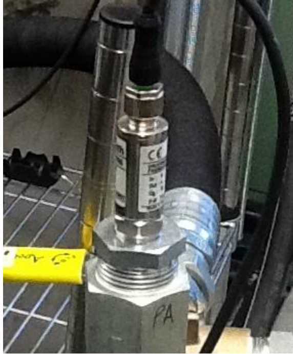
Figure 55: Pressure transducer (center) is connected to the data acquisition system via electrical cabling, which attaches at the top of the unit.
