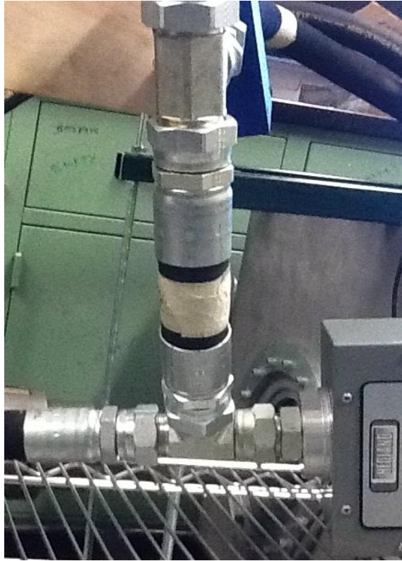
Figure 64: Flow to the left (out of the Hedlands flow meter) through H8 (bottom left) goes to the 10 bar check valve. Flow upwards, through H16, follows the main circuit (center).
