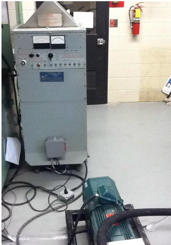
Figure 63: Load bank (upper left) is attached to the generator (lower center) via electrical cabling.
