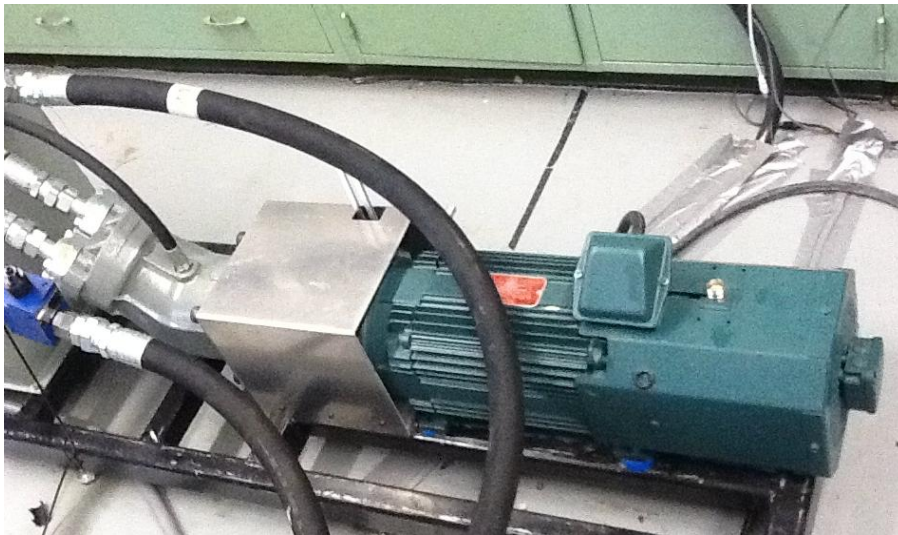
Figure 62: Axial piston motor (far left, gray) is attached to the generator (center, green) via the second set of couplers.
