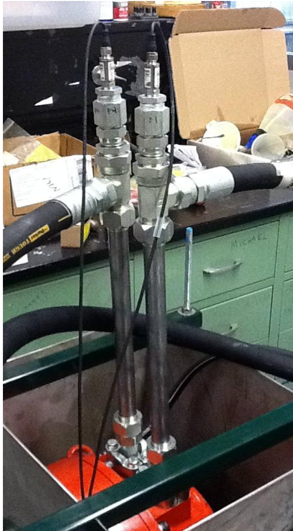
Figure 60: 18" pipes, center, allow both outlet and inlet ports of the Hagglunds pump to clear the sheet metal enclosure tank.
