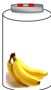
Figure 13: Closed jar system used for 1-MCP treatment
