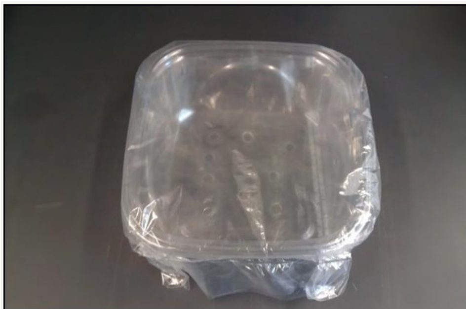
Figure 14: Permeable package system used for 1-MCP treatment
