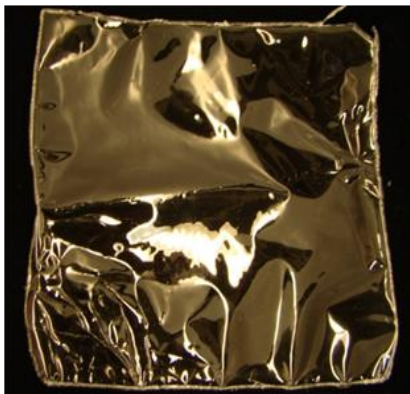
Figure 30: PVA film obtained using casting method
