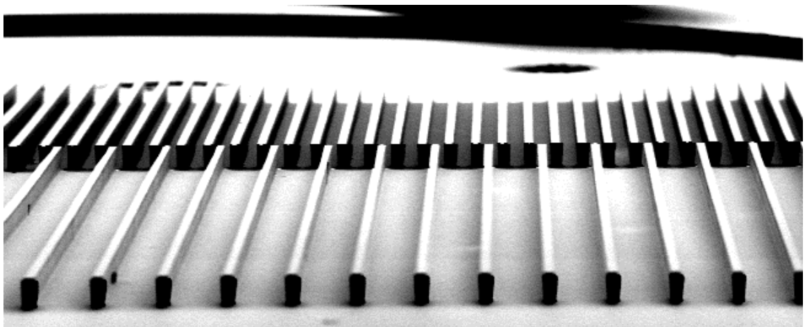
Figure 2.3. Fabrication and packaging process of microchannel heat sinks (Plasma Etching).
