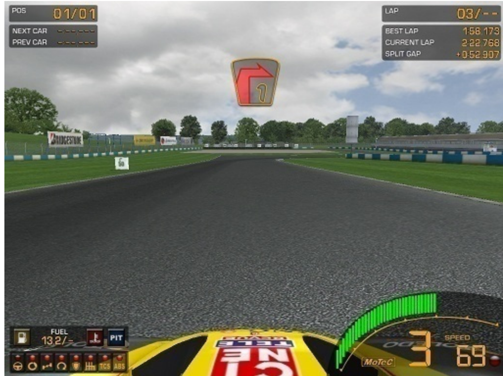
Figure 4. Depiction of driving aide arrow. This aide was available during practice and experiemental sessions. The figure above shows a Red Arrow pointing to the right containing the number one. This indicates that a difficult right turn is approaching in approximately one second. If the arrow were yellow, pointed to the left and contained a 3 that would mean that an easy left turn was approaching in approximately 3 seconds.
