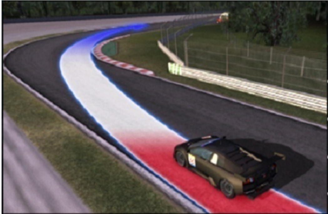
Figure 3. Depiction of the “driving line” available to participants during practice driving sessions. Red indicated a need to apply brakes, blue stressed acceleration and white suggested neither braking nor accelerating.
