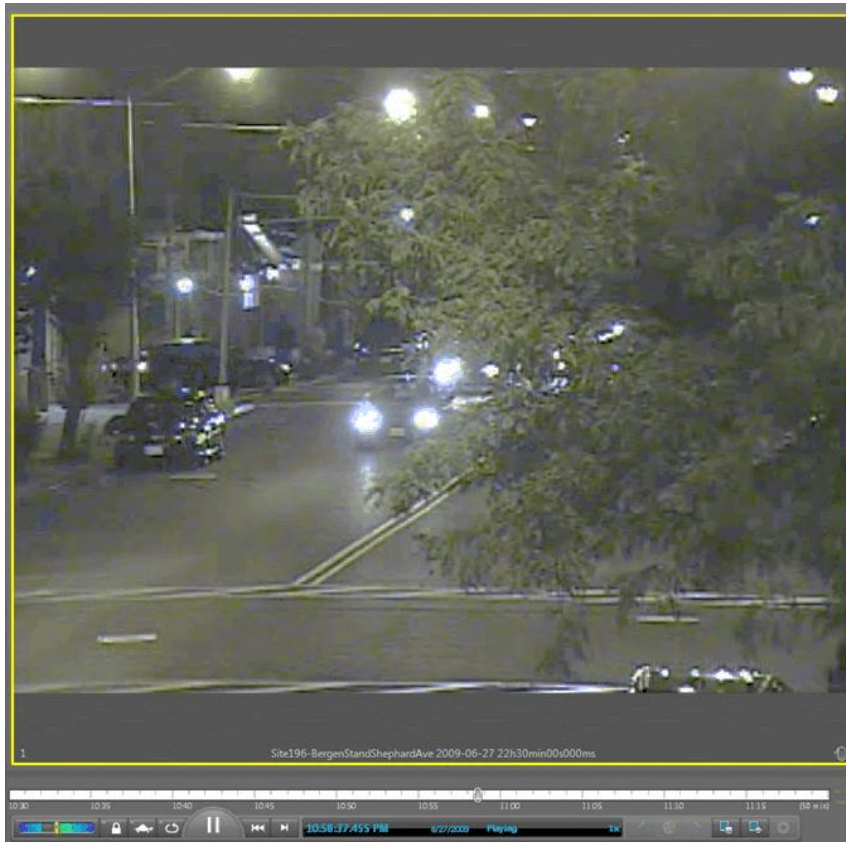
Figure 11: Leaves from a tree obstructing the view of a camera.
