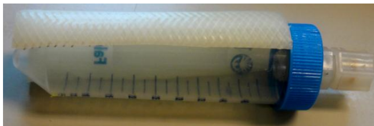
Figure 6: Setup of insulated falcon tube which was filled with peanut butter and fitted over two thermocouples of HHPP unit
