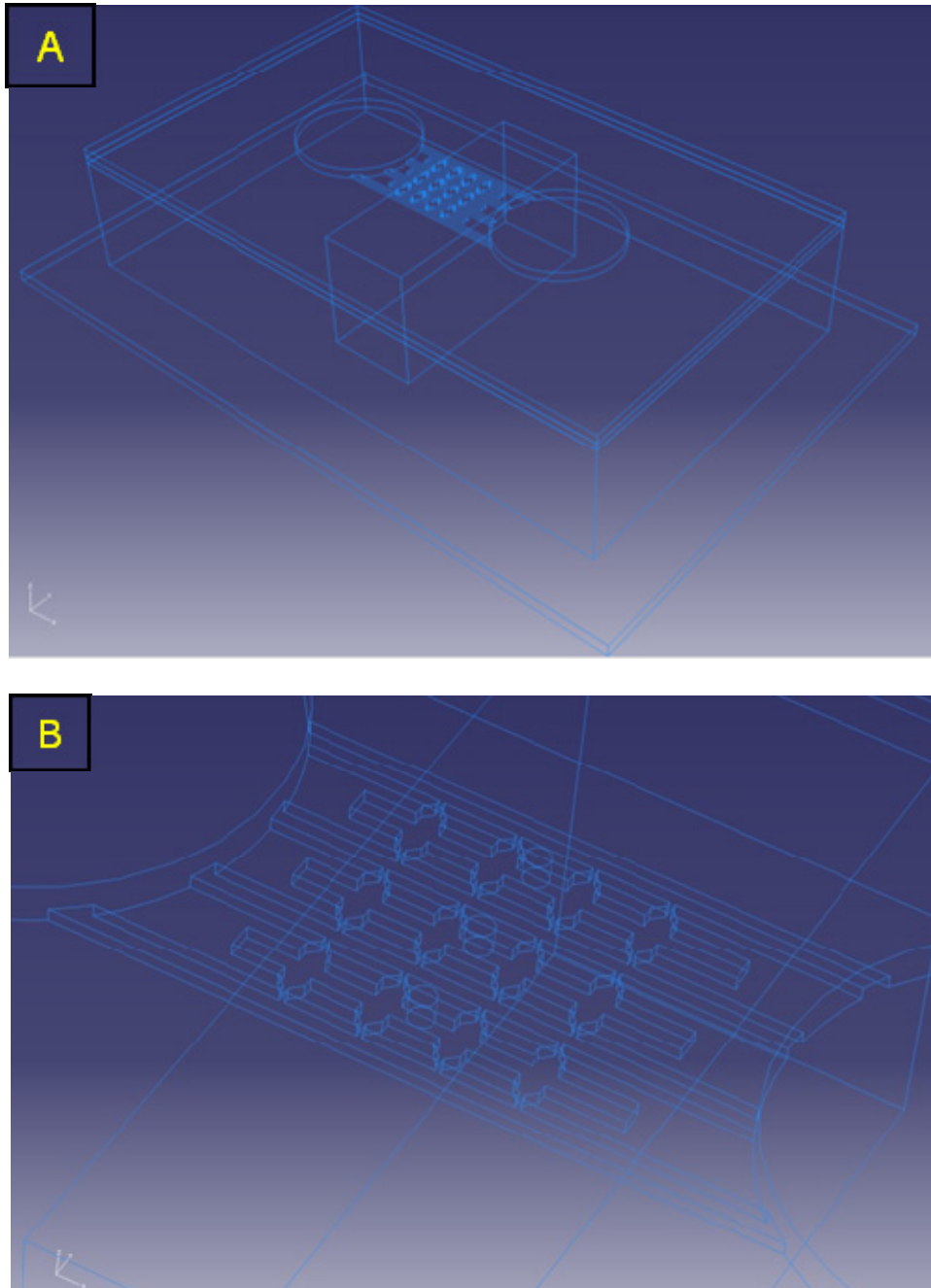
Figure 4.2. Schematic of a potential device that allows for the incorporation of oligodendrocytes. A) Isometric view of proposed device showing different PDMS layers on a glass coverslip. B) Detailed view of central microchannel portion of the device, showing long channels connecting two mini-wells and oligodendrocyte inlet ports (channels and ports not to scale).
