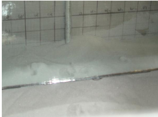
Figure 46: Fluidized bed surface above a disk submerged 0.76R deep
