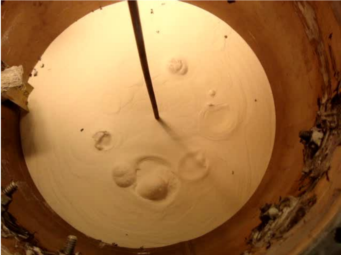
Figure 57: Bed surface picture of sphere of radius 0.03334m submerged 4.1R in fluidized bed of \text{Al}_2\text{O}_3 . Voids outline the perimeter of the submerged sphere.
