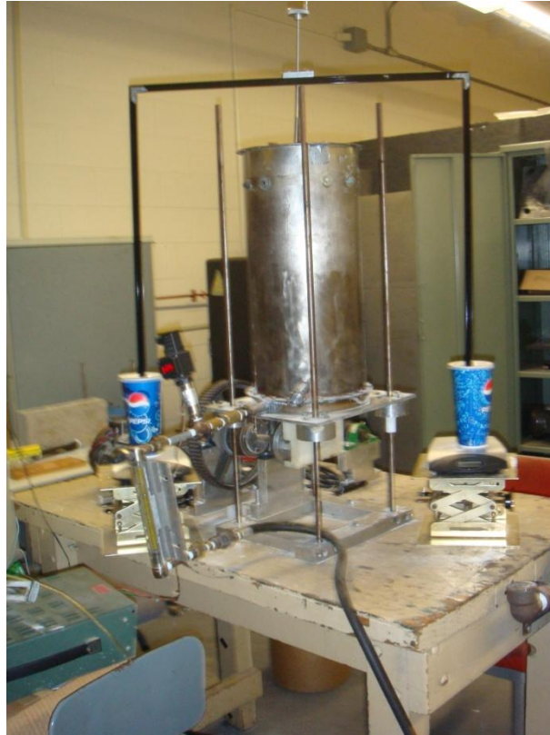
Figure 35: Photograph of assembly for measuring forces on submerged objects shown inside bed
