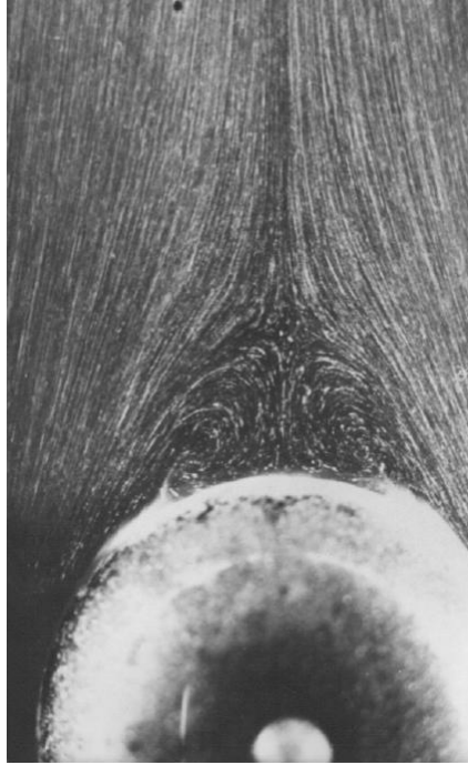
Figure 26: Flow past a sphere at Re = 37.7 . [Taneda 1979]
