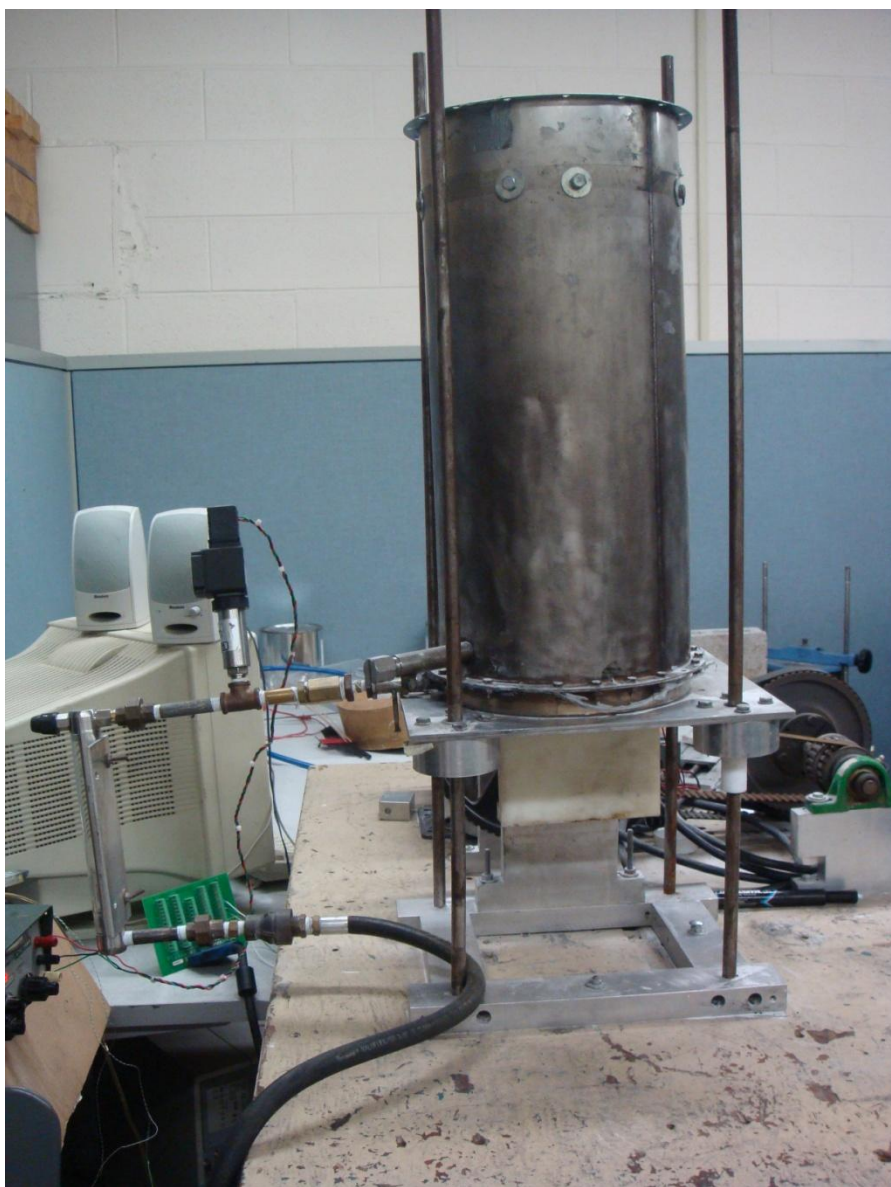
Figure 31: Photograph of fluidized bed set-up
