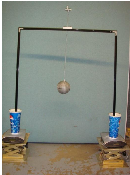
Figure 34: Photograph of assembly for measuring forces on submerged objects shown outside of bed
