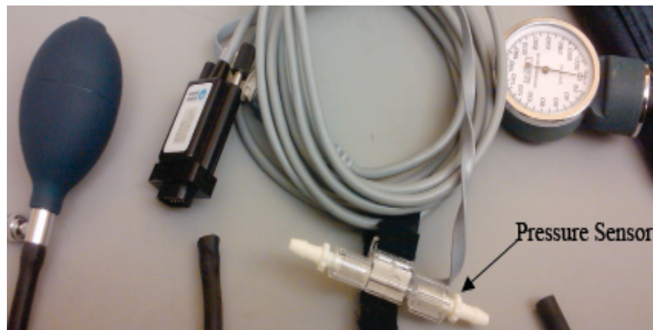
Figure 10: Biopac™ pressure sensor taken apart from pressure cuff and bulb.
