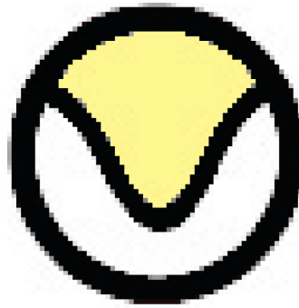
Figure 7: Cross-sectional area of the plaque dome models representing a plaque dome formed on the upper wall and a remaining lower flexible wall.
