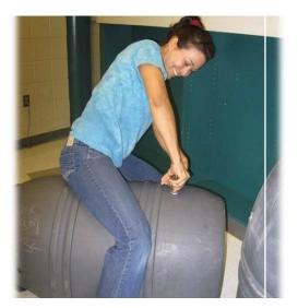
Line-up the threaded portion of the faucet with the hole in the barrel, and applying pressure, screw in the faucet. The sealant will pile up behind the faucet as you screw it in, filling in any small cracks.
