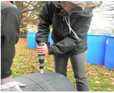
**Faucet:** For a screw top barrel, use the drill and one inch hole saw to drill a hole about six inches up from the bottom. If using a closed top barrel, the length of your reach inside the barrel to where you can screw on the lock nut will determine how far down the hole should be drilled. Avoid drilling on a seam, which will cause the barrel to crack and leak.
