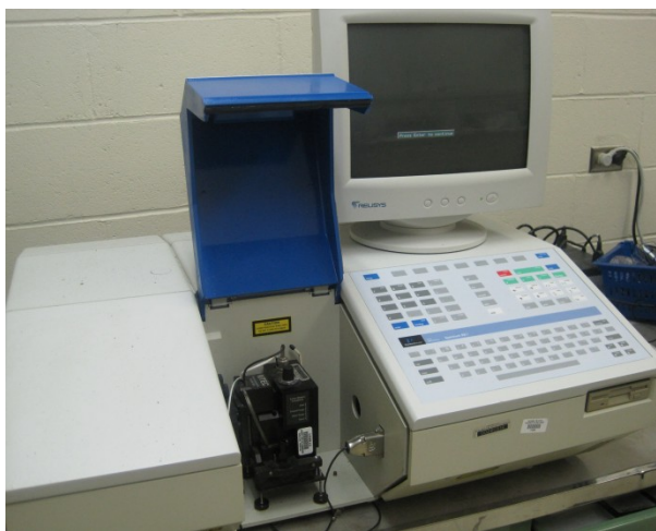
Figure 22. The Perkin Elmer Spectrum RX I FTIR spectrometer and MTEC model 300 photoacoustic detector.
