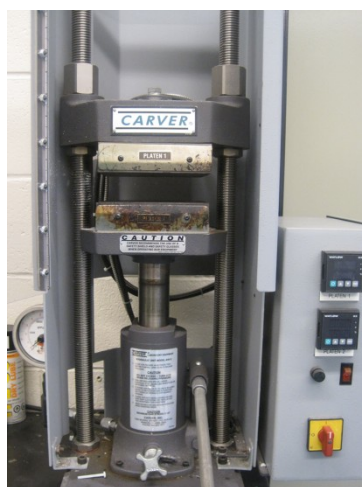
Figure 8. The Carver® compression molding press.
