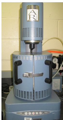
Figure 10. TA Instruments, AR-2000 parallel plate rheometer.
