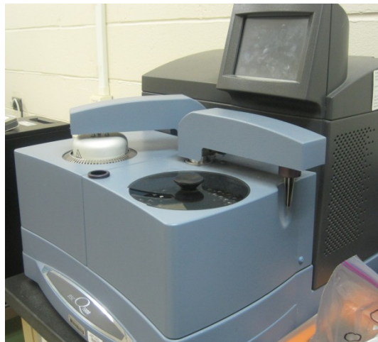
Figure 25. TA Instruments DSC Q1000 equipment.
