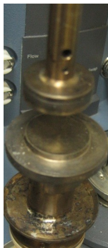
Figure 11. Parallel plate geometry of the AR-2000 rheometer.
