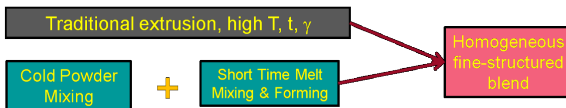
Figure 3. Illustration of the conventional extrusion method in comparison to the two part powder processing method resulting in the same homogeneous, fine-structured blend.
