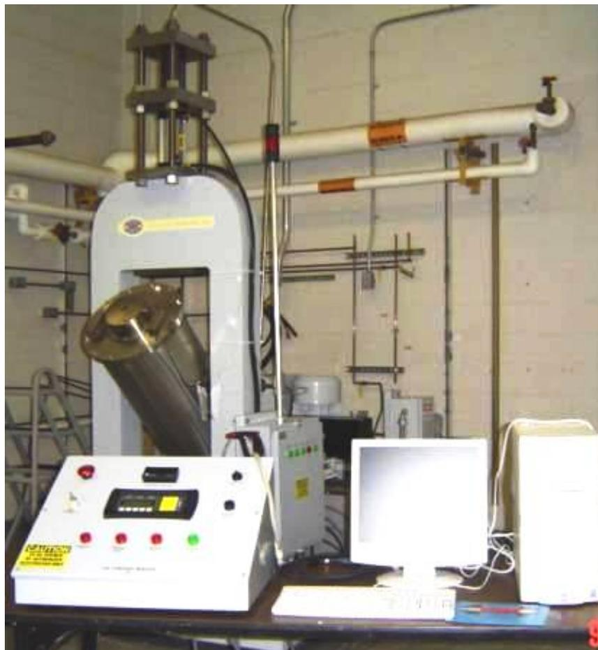
**Figure 4-1: Rutgers 10 liter high hydrostatic pressure processing facility.**
