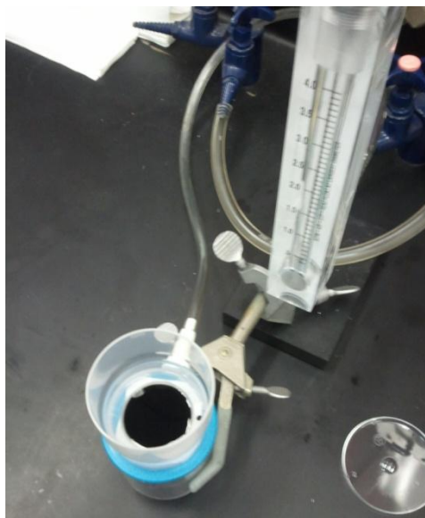
Figure 4-9: Pressure induced wetting set up. Apparatus includes a 0.2 micron filter connected to a flow gauge and vacuum line.
