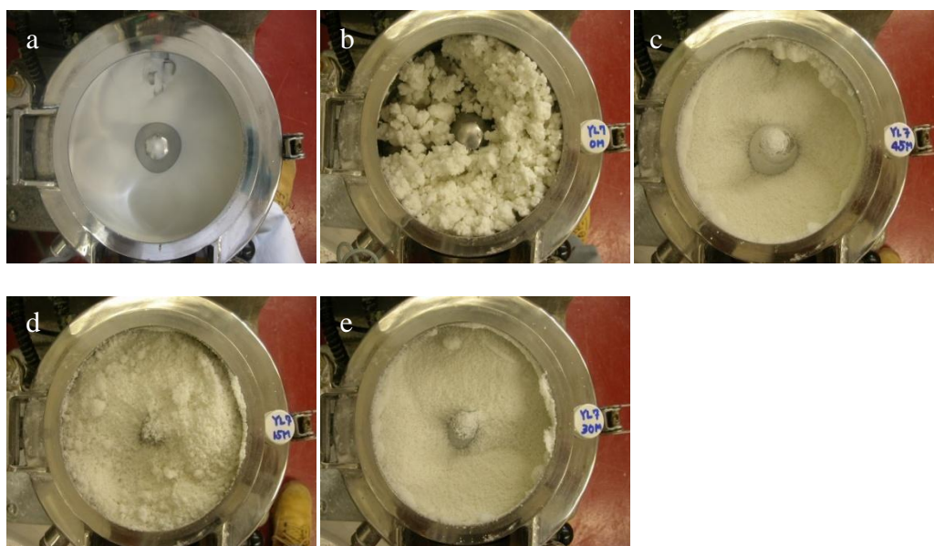
Figure 5-3: View of the Fukae granulation as a function of time. (a) powder only (b) 0 minutes (c) 15 minutes (d) 30 minutes (e) 60 minutes.
