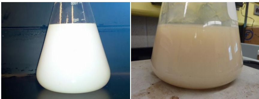
Figure 6-4: Sol-gel of alumina (left) and after mixing with graphene oxide (right).
