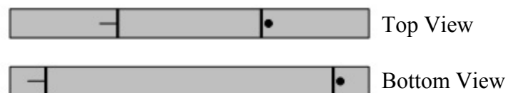
Figure 4.5 Bend bar labeling diagram. Positions of loading pin contact zones and bar orientation marks where marked on the top and bottom surfaces of each bend bar
