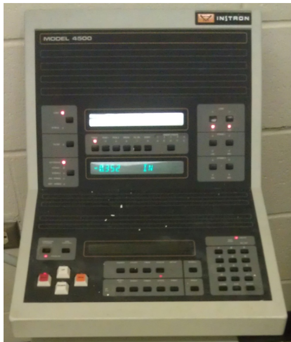
Figure 4.7 Instron 4500 Test Frame Control Board. Allowed for manual operation of crosshead and measurement of applied load
