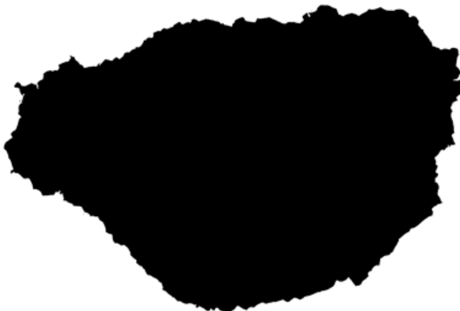
Figure 5.102 Porous boron carbide inclusion on polished section of SiC flexure bar. Image has been converted to binary. Filled area corresponds to visible cross section of inclusion
