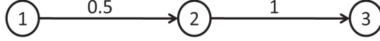
Figure 3.7: A three node network with linear topology. Node 1 tries to deliver 100 packets to node 2 and node 3.
