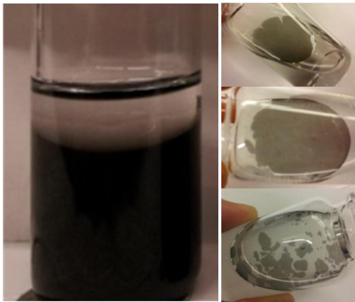
Figure 4.5: Digital photographs of: (left) ME-LOGr suspension with toluene added and the same system with (from top to bottom) 1 mL, 2 mL and 5 mL of additional ethanol.
