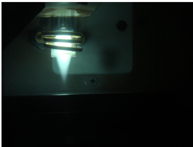
Figure 3.4 Plasma generated by a 40.56MHz ICP.
