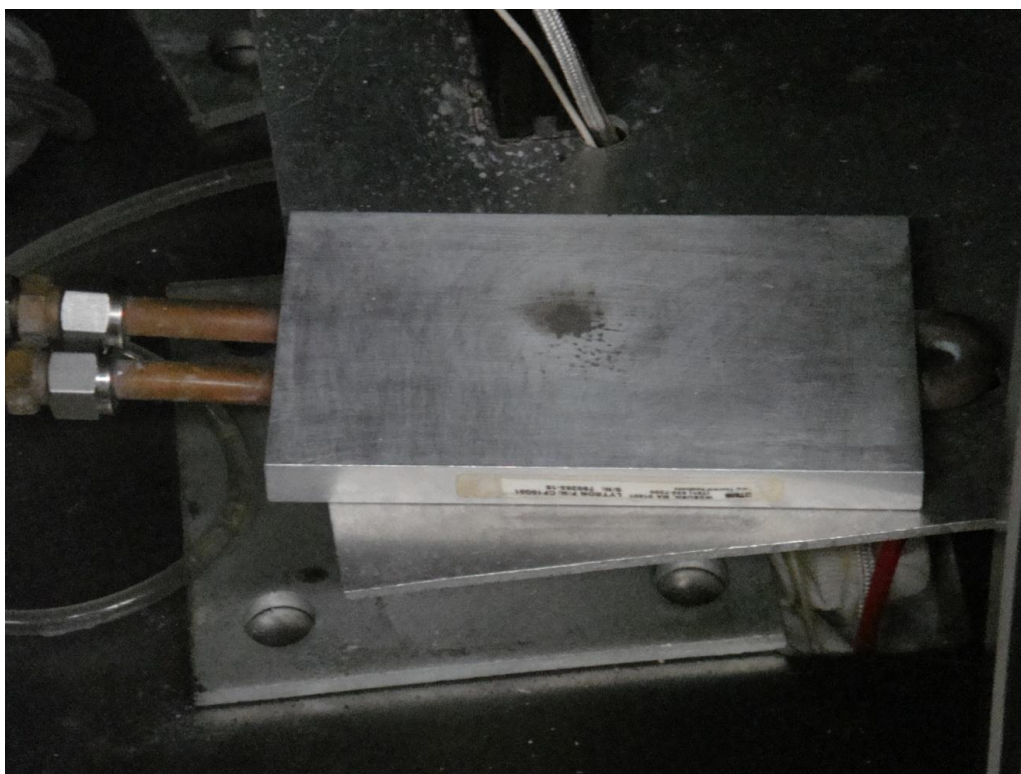
Figure 3.8 Aluminum substrate used to collect as-synthesized nano-particles.
