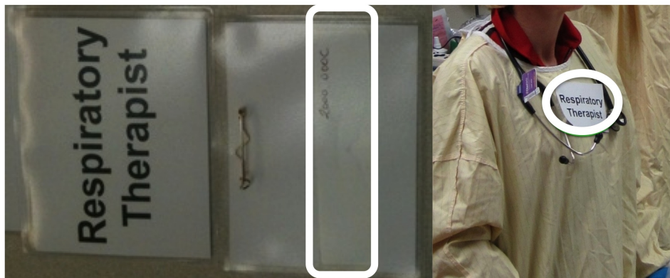
Figure 6.12: Front and back views of a role tag. The RFID tag is attached on the backside.
