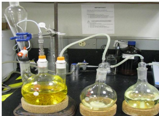
Figure 12. Preparation of chlorine dioxide stock solution
