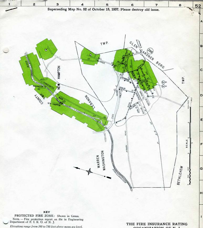
Elevations range from 340 to 780 feet above mean sea level. Water mains 8 inches and larger in diameter Water mains 6 inches in diameter Water mains 4 inches in diameter Fire hydrants shown thus
