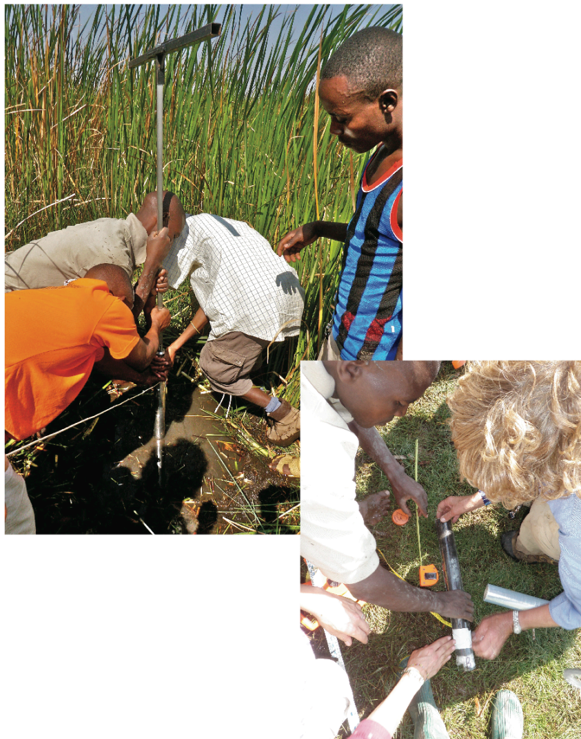
Figure 10. Upper image: field assistants pushing corer into the ground to collect Core 1A. Lower image: Core 1A has been extruded and encased in core liner and is being wrapped and secured for transport.
