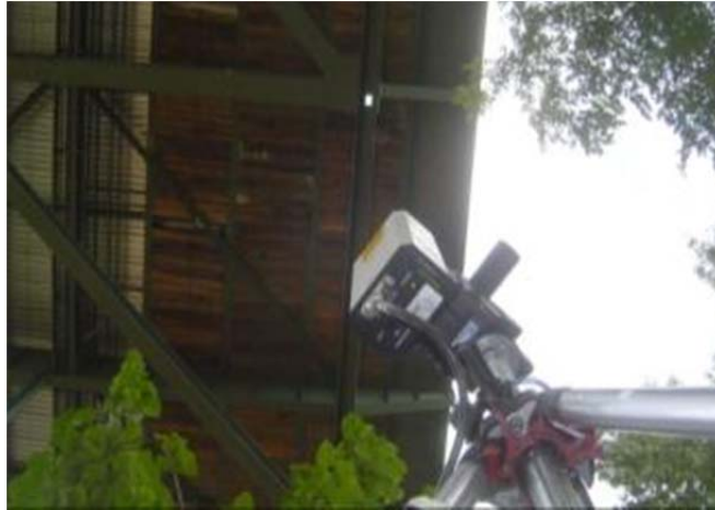
Figure 3.4 Polytec PI Laser Doppler Vibrometer (LDV) underneath the Hackensack River Bridge
