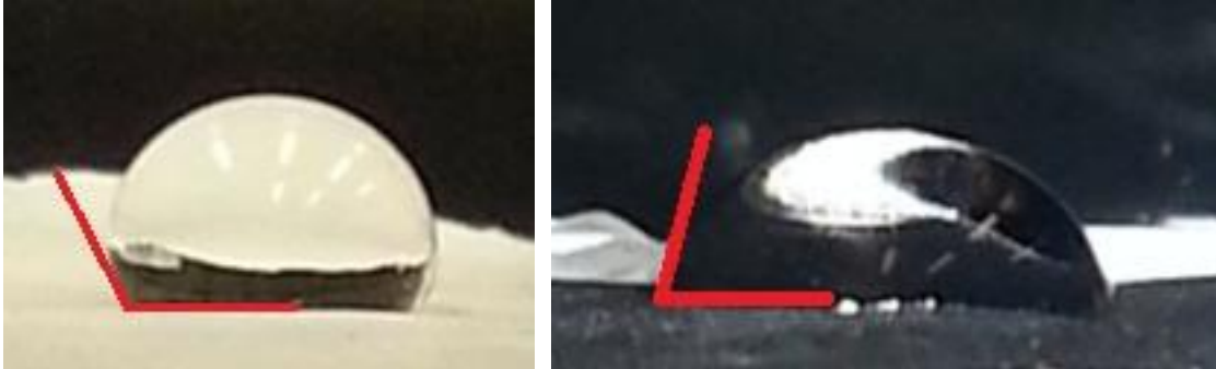
Figure 2-9: Contact angles for PLGA (left) and SWNT-PLGA (right) scaffolds with a contact angle of 117 and 80 degrees respectively.
