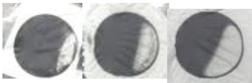
Figure 2-12: Gradient scaffolds impregnated at 5.5°, 11°, and 15°.
