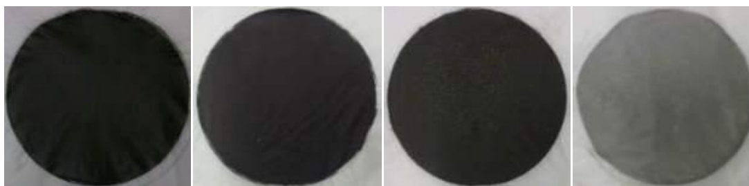
Figure 2-6: Vacuum impregnated scaffolds with dispersions of varying CNT concentrations of 0.4%, 0.2%, 0.1% and 0.05% from left to right.
