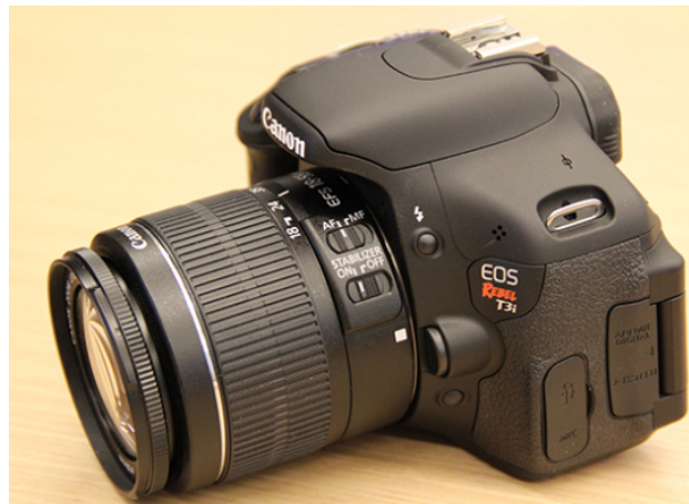
Figure 2.2: Canon EOS Rebel T3i. Two such cameras are used for surface imaging of bridge decks.
