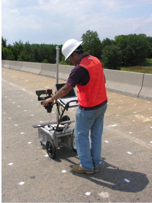
Figure 4.3: Initial stages of test, where the cart was used for image collection.
