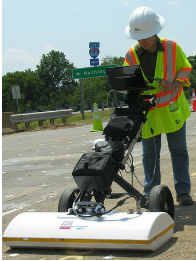
Figure 1.3: Ground Penetrating Radar used to detect subsurface corrossions [3]. Courtesy: Dr. Nenad Gucunski
