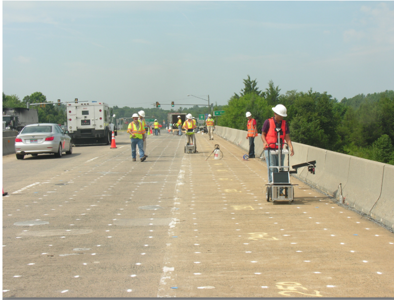
Figure 1.2: Various inspection processes being carried out on-field at the Virginia testing site. These include ground penetrating radar, resistivity, surface imaging and impact-echo tests. The white dots seen in the image are the grid-markings. Courtesy: Dr. Nenad Gucunski
