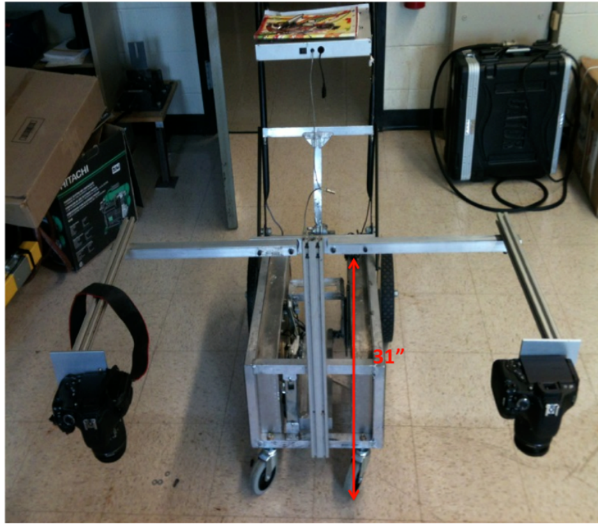
Figure 3.5: Front view of the mounting system showing the distance between the ground and the arms.
