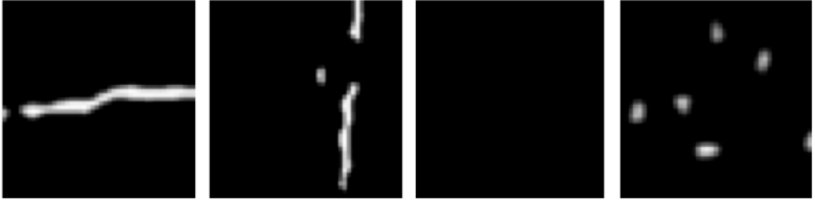
Figure 4.27: The four patches correspond to four regions: horizontal crack, vertical crack, no crack and noise. The area of the white regions in the patches is used as a feature for classification.
