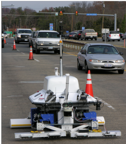
Figure 1.4: Bridge inspection robot with various systems mounted on it. It reduces manual labor by a considerable amount. Courtesy: Dr. Nenad Gucunski
