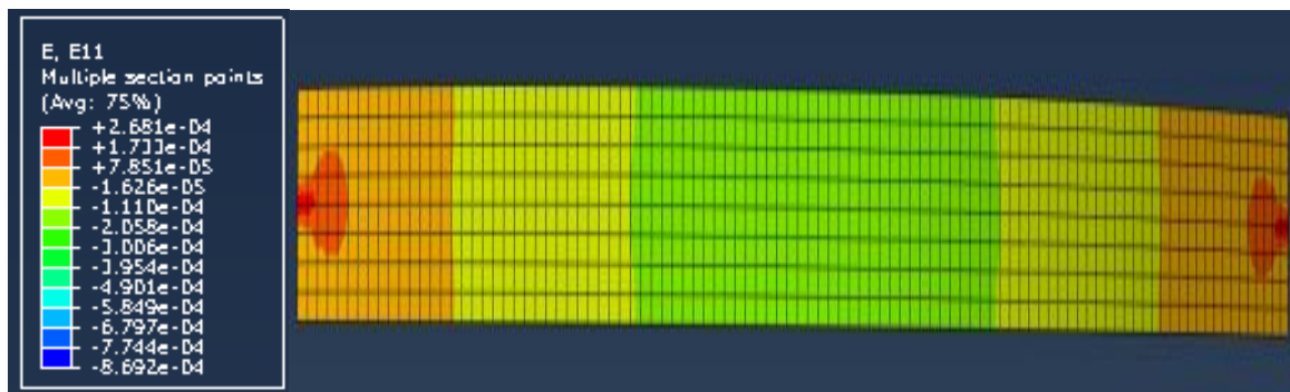
Figure 55: Shrinkage in top of the deck for 10 in thickness of deck
